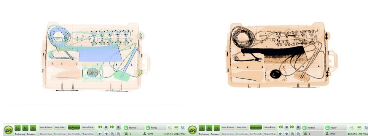
Figure 5 - High Penetration (5030A right side)
