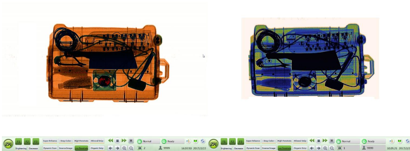
Figure 6 - Low Penetration (5030A right side)
