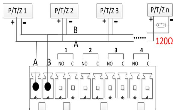
PTZ's "+" terminal should be connected to DVR's interface "A".
