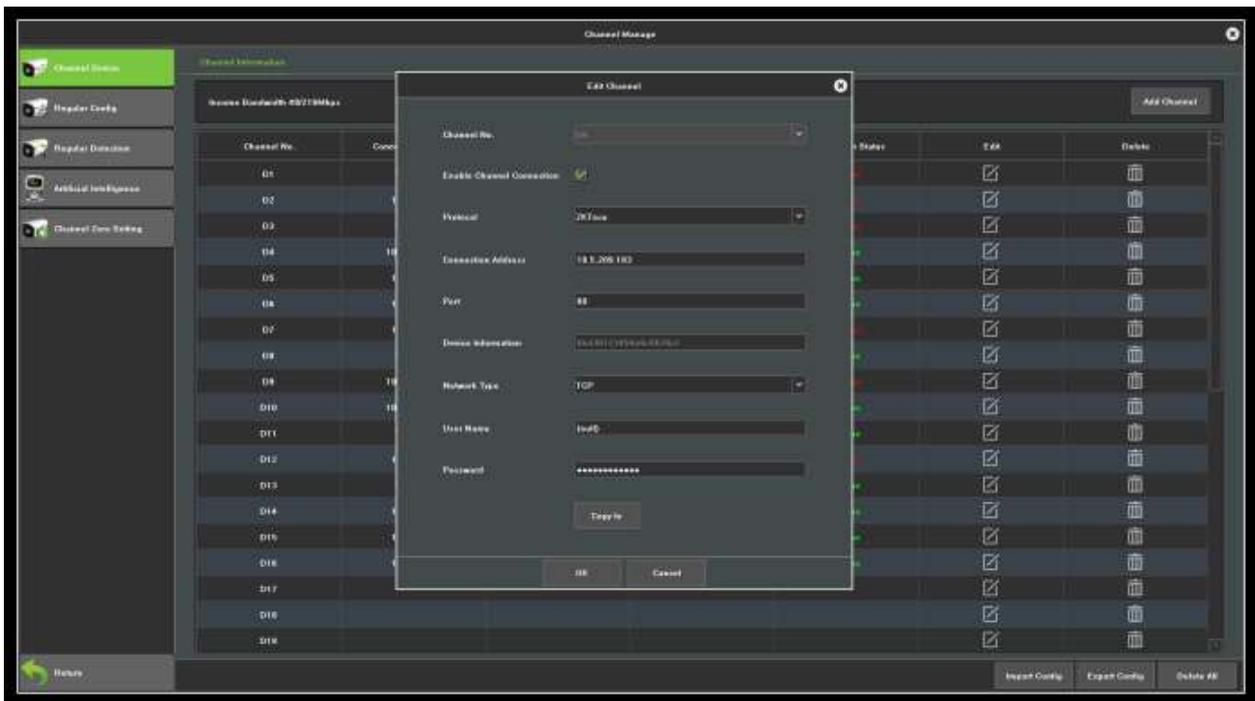
Figure 7.2 Custom Adding IP Camera Interface
