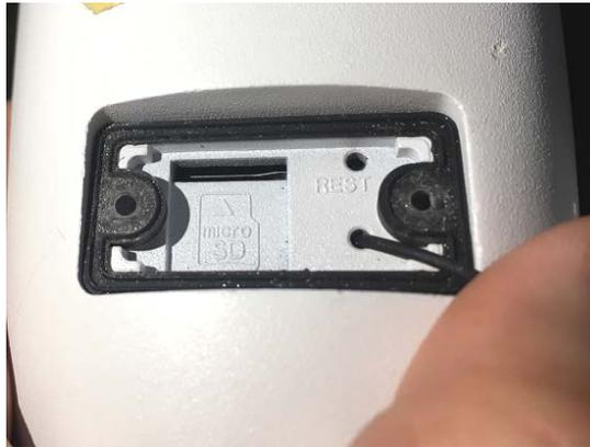
**Step 3, install the Micro-SD card in the correct direction and insert it into the slot.**
