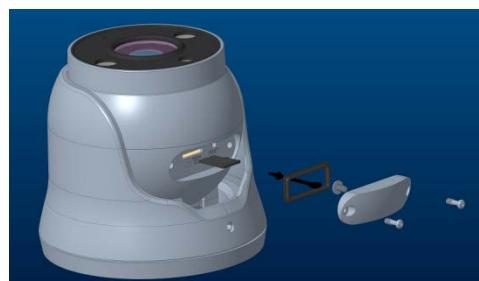
**Step 4, close the cover and tighten the screws.**
