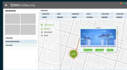
According to the plan, the video is played sequentially on the map and the Check in button appears randomly to avoid malfeasance of the patrol staff
