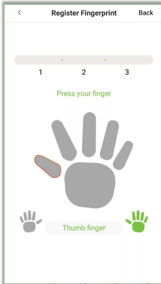
2. Press the same finger on the fingerprint reader three times. The Green bar indicates that the fingerprint was registered successfully.
