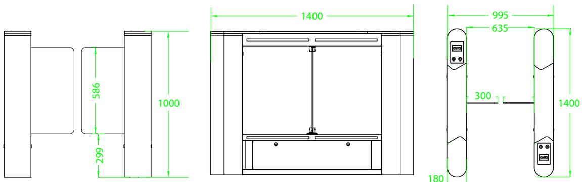
\* Turnstile can work in the temperature of -20°C to 70°C. If the temperature is under -20°C, acrylic parts may be broken. (Temperature control device is optional to solve this problem.)
