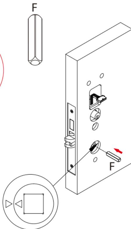
**Note:** Ensure the two triangles are in horizontal alignment.
